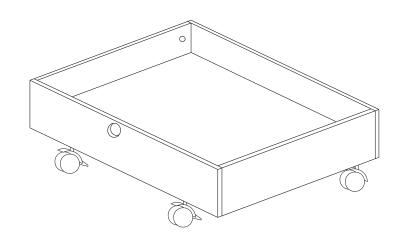
Attach 2x wheels (E) and 2x wheels (F) to the underside of the box as shown, using 16x screws (D). Tighten with a screwdriver.
