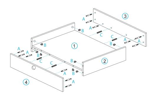
Attach the two side panels [2] to the base panel [1] with 4x bolts (A), 4x dowels (C) and secure with 4x locking nuts (B). Tighten with a screwdriver.
